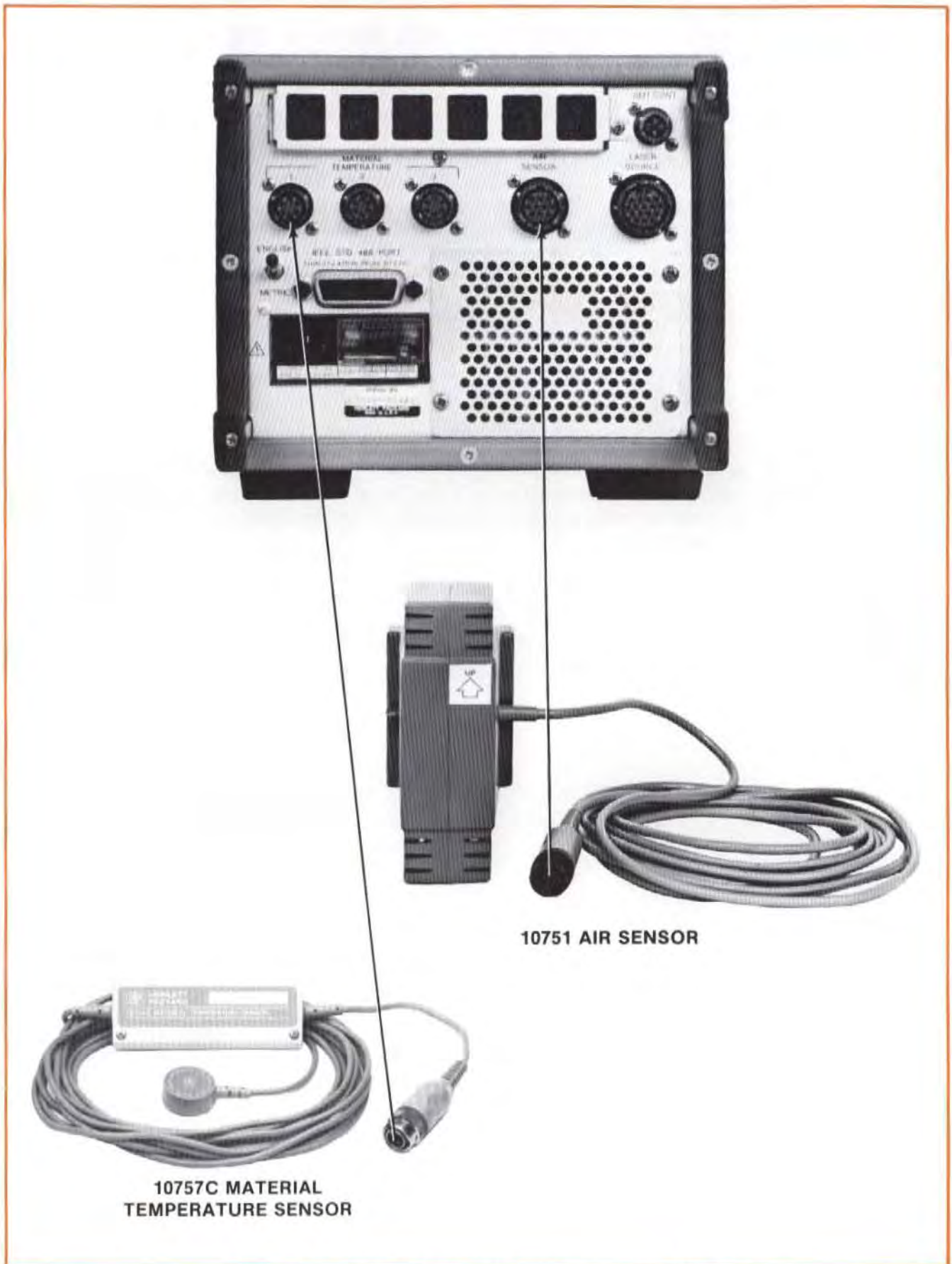
Figure 5-2. Connecting Sensors to the Measurement Display
