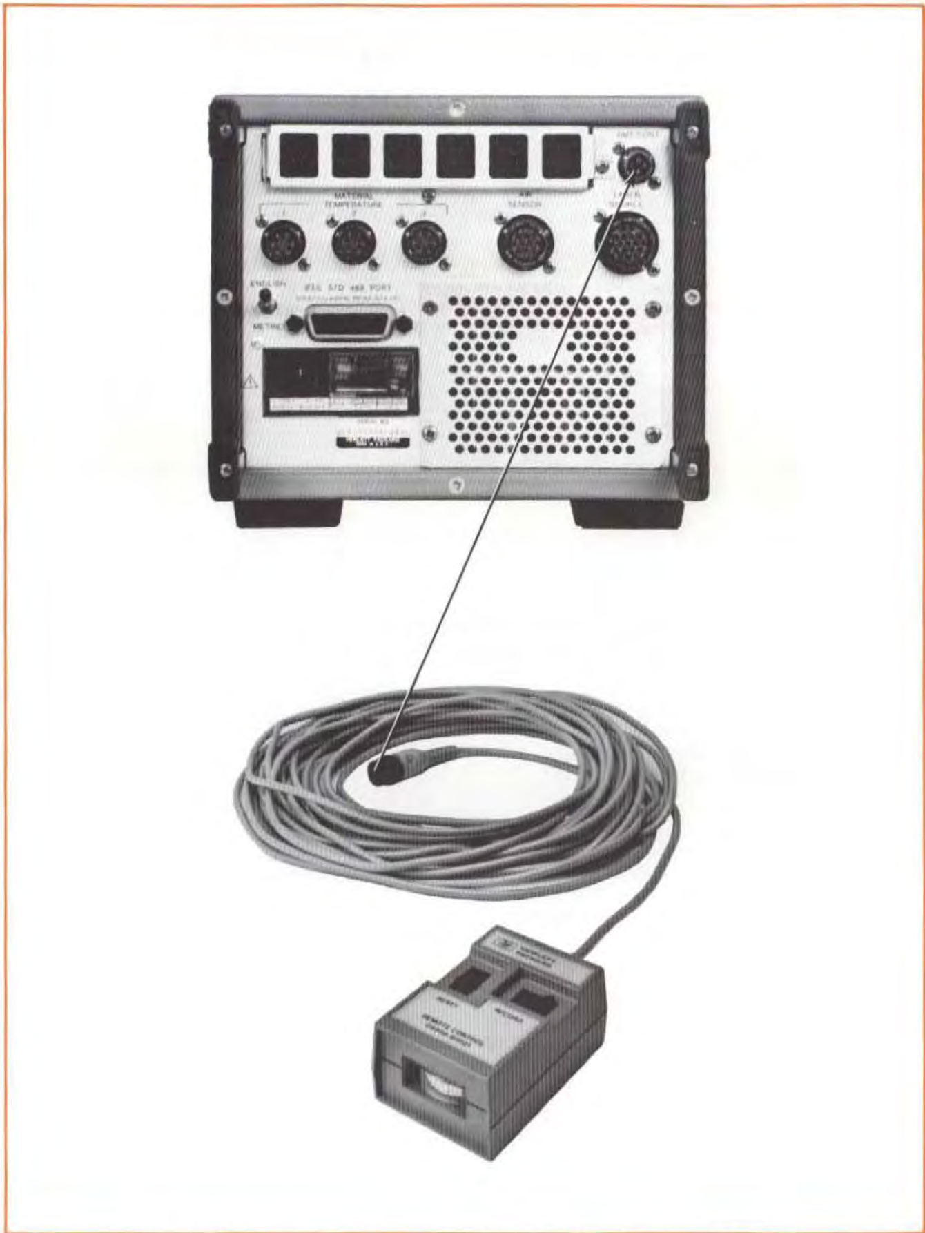
Figure 5-3. Connecting the Remote Control Box to the Measurement Display
